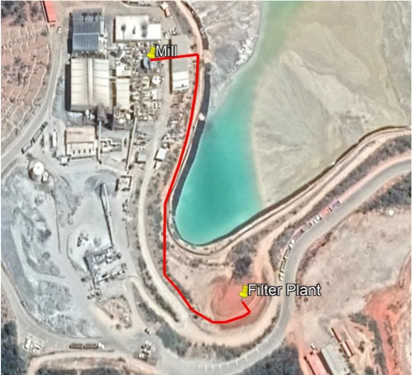
Figure 10-31: Pipeline Route for Filtered Tailings Feed Pipeline.
